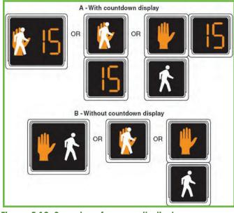
Figure 5.10. Samples of crosswalk displays.
