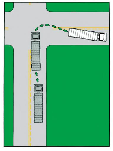
This illustration shows how to make a right turn with a tractor semi-trailer. If the turn is sharp or difficult, swing out into the street you're about to enter. Watch the off-track to avoid running over the curb.
