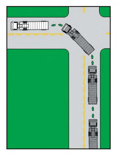
This illustration is the correct procedure for making a left turn with a tractor semi-trailer. The procedure is the same with a single-unit vehicle.
