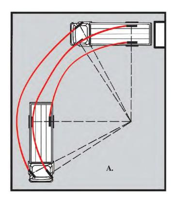
A. Steering (backing) with a single-unit vehicle
